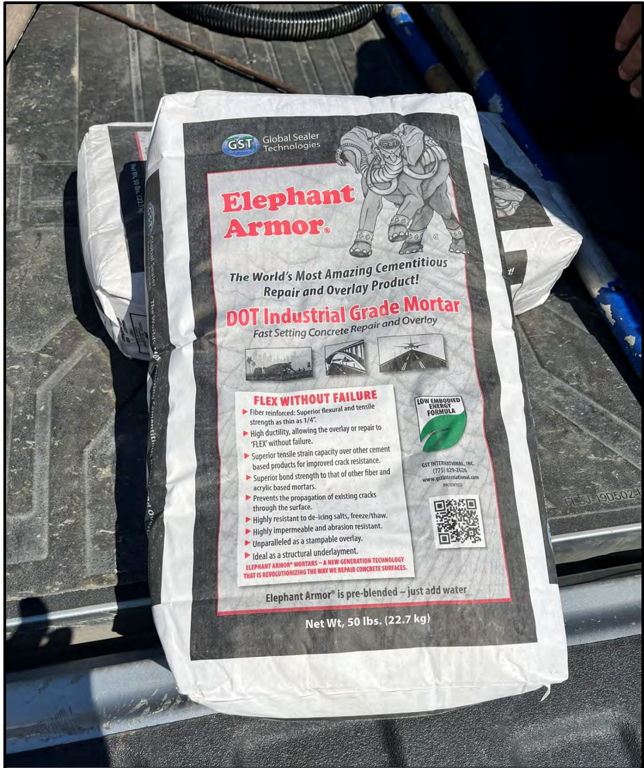
Elephant Armor joint sealant used to fill the gaps in the pipe joints and the cracks inside the manhole.
